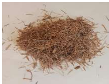
Fig 3 Coconut Coir Fiber used in reinforcement phase
